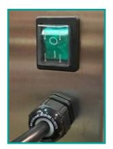
Screw the hose connector into the drain valve located on the rear of the unit.
