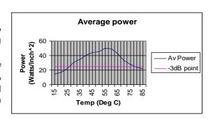
Ultrasonic activity itself will heat up the liquid at a rate of approximately 10-15°C per hour if in continuous use.
