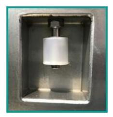
If there is insufficient fluid in the tank to activate the float level sensor, the digital control panel will display the scrolling message "LEVEL".
