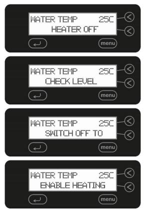
To continue using your Qi-Series ultrasonic bath, refill with liquid up to the level sensor, switch the unit off and on again.
