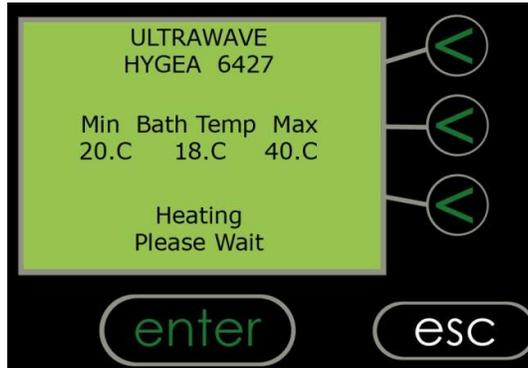
The **Hygea 6427** will automatically start heating and degassing the liquid.
