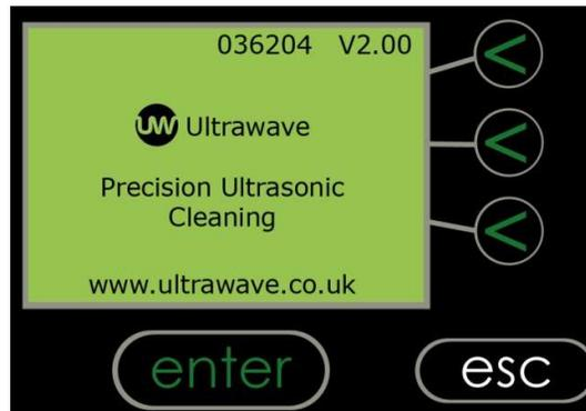
While this screen is displayed, the buttons are inoperative. This is normal as the **Hygea 6427** is running through its start-up routine and checking all internal systems are working correctly.
