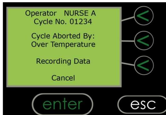
If the liquid temperature drops below the pre-set minimum temperature during operations, the cleaning cycle will stop and the following screen will display:
