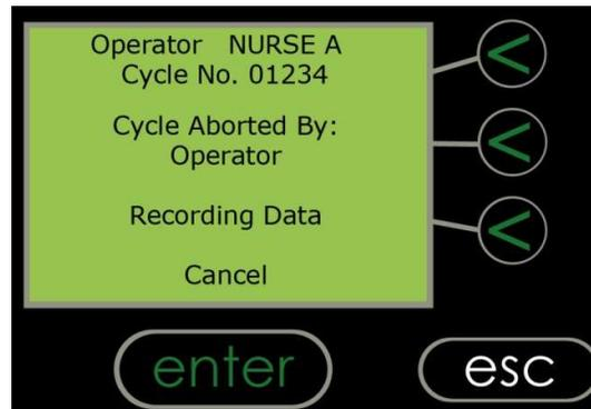
If the fluid level drops below the required level during operation, the cleaning cycle will stop and the following screen will be displayed:
