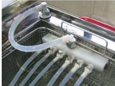
2. Connect the basket by inserting the connector into the luer located on the top of the tank.
