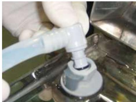
3. Connect the other end of this hose to the manifold located on the basket.
