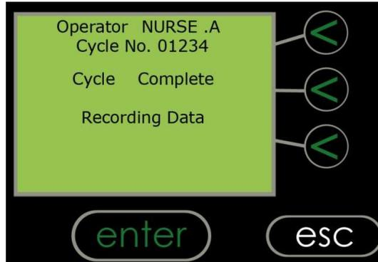
If the print option is chosen, then at the end of each cycle, the integral printer in the **Hygea 6427** will print a ticket showing the details of that cycle:
