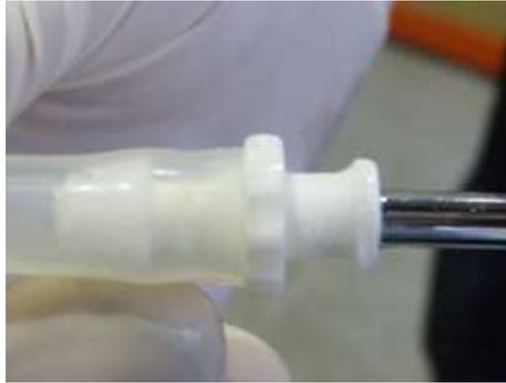
5. The instrument and hose can then be connected to the manifold.
