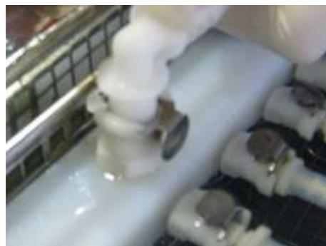
4. The instruments can be connected by inserting the correct size connector into the tube and then connecting the hollow instrument.
