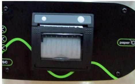
**Step 7** – Feed a small amount of paper through the printer by pressing the paper advance button on the right hand side of the printer or the paper button on the panel.
